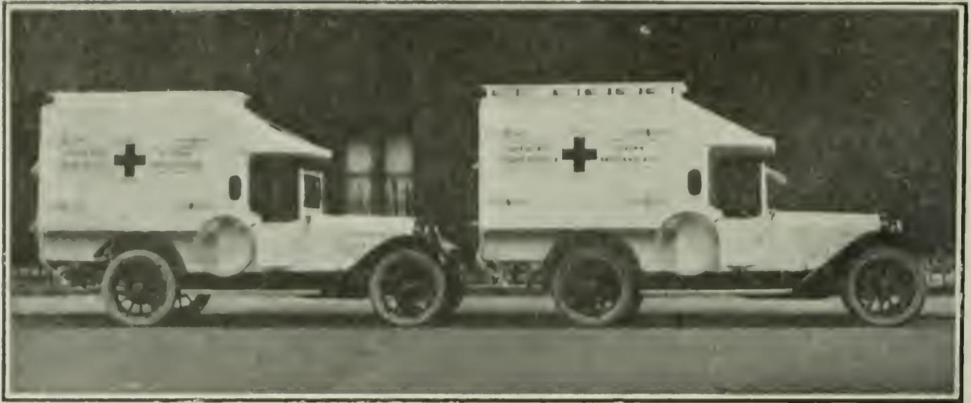
MOTOR AMBULANCES FOR EAST AFRICA With ventilated roofs and sides.
