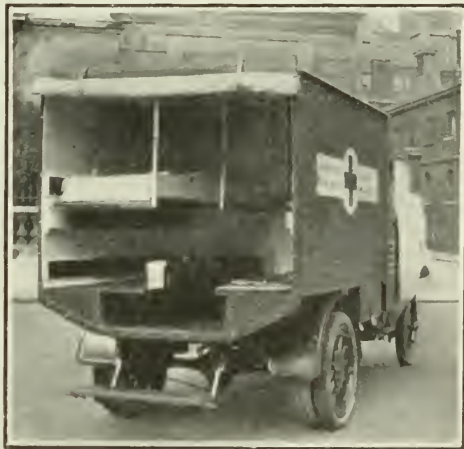
MOTOR AMBULANCE FOR NAVAL USE, Fitted for cots instead of stretchers.
